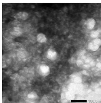
Fig. 2 TEM image of SLN-Famotidine. Scale bar: 100 nm.
