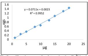
Fig(2): calibration curve for determination Zn<sup>2+</sup> ion in aqueous solutions by dithiazone method.
