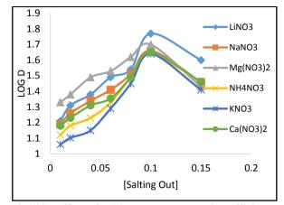
Fig (20): effect of salting out on extraction efficiency and D-values
