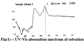
Fig(1) = UV-Vis absorption spectrum of solvation species The spectrum show  $\lambda_{max}$ =291 nm was the wave length of maximum absorption for solvent species of  $Zn^{2+}$  ion
