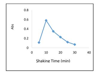
Fig(7): Effect of shaking time on formation and stability of solvation species
