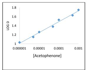
Fig(10): effect of acetophenone conc. On Extraction efficiency and D-Values
