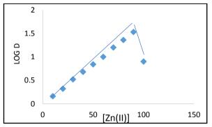
Fig (6): Effect of Zn<sup>2+</sup> ion conc. On extraction efficiency and D-Values
