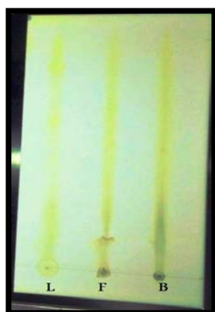
Figure 2: Thin layer chromatography for phenol extracts , system n-butanol: acetic acid: water (4: 1: 5) (L: leaves , F: fruit , B : bark).
