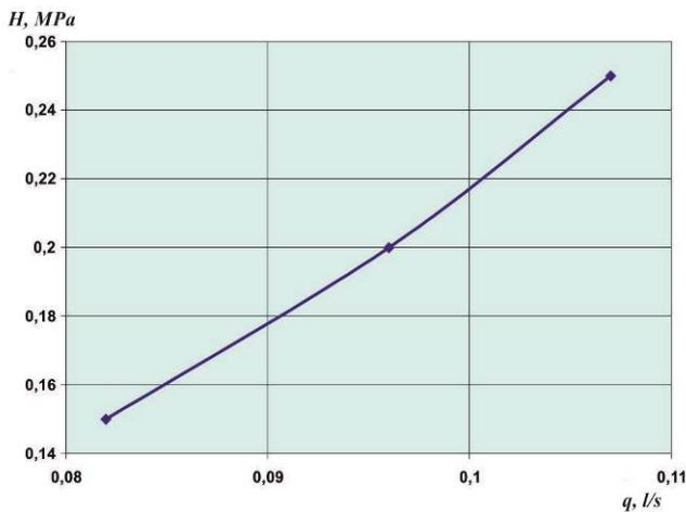
**Figure 6 – Rate and head-flow characteristic of carousel nozzle**
