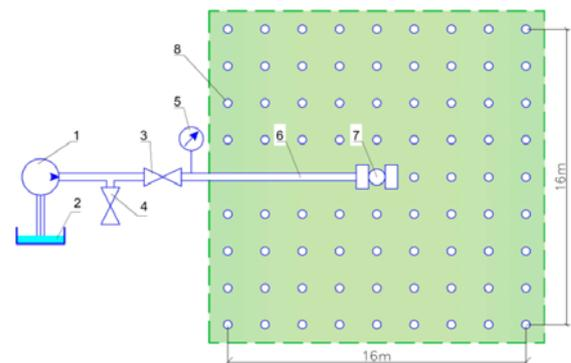
**Figure 3 – Principal diagram of the stand for identification of the parameters of sprinkling nozzles: 1 – pump; 2 – accumulation tank; 3 – tap; 4 – pressure regulation valve; 5 – manometer; 6 – piping section; 7 – sprinkling nozzle; 8 – rain-cups**
