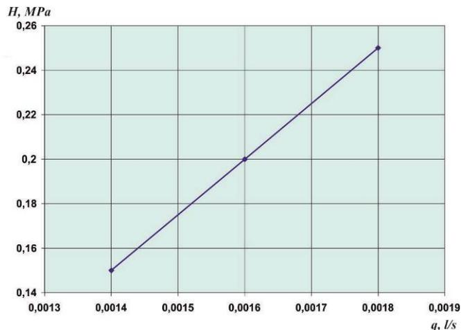
**Figure 7 – Rate and head-flow characteristic of sprinkler nozzle**
