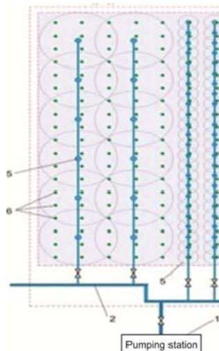
**Figure 5 – Diagram of the bench site for testing the modular mist sprinkling systems: 1– pumping station; 2 – distribution piping; 3 – sprinkling piping; 4; 5 – sprinkling nozzles; 6 – fruit trees**
