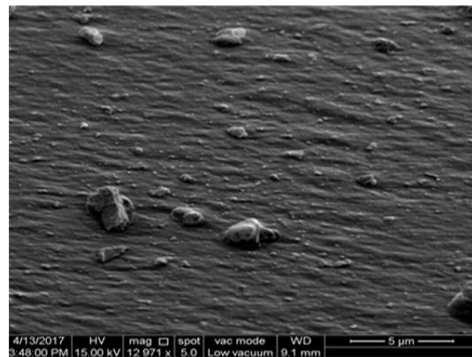
Fig. 3: SEM micrograph of biogenic silver nanoparticles. The shape of AgNPs was spherical and homogenous, size between (64-100nm).
