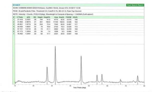
Fig.2 : XRD analysis of Biosynthesized nanoparticles using *P.agglomerans* (average diameter 16.73nm)
