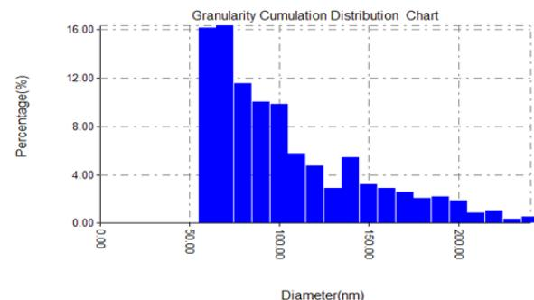
Fig.5. Atomic Force Microscopic analysis of biosynthesized silver nanoparticle from *P.agglomerans* (Average Diameter: 98.78 nm)
