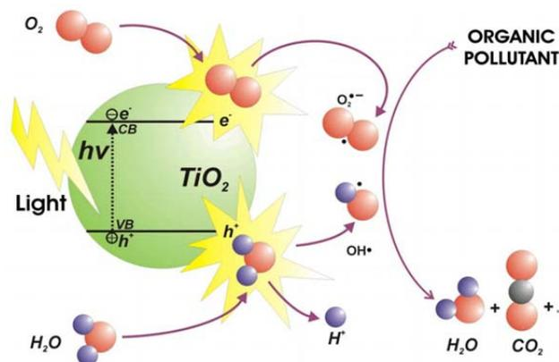
**Scheme 1.** Graphical of semi-conductor excited through energy gap enlightenment [16] major to electrons induction in band of conduction with the valence band holes.
