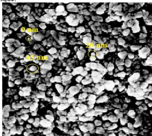
**Figure 4,** The SEM picture of TiO<sub>2</sub> nanoparticles
