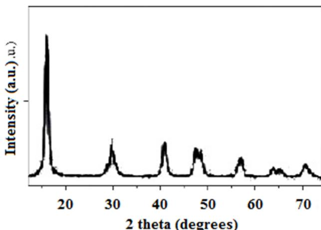
Figure 5, The XRD of TiO<sub>2</sub> nanoparticles
