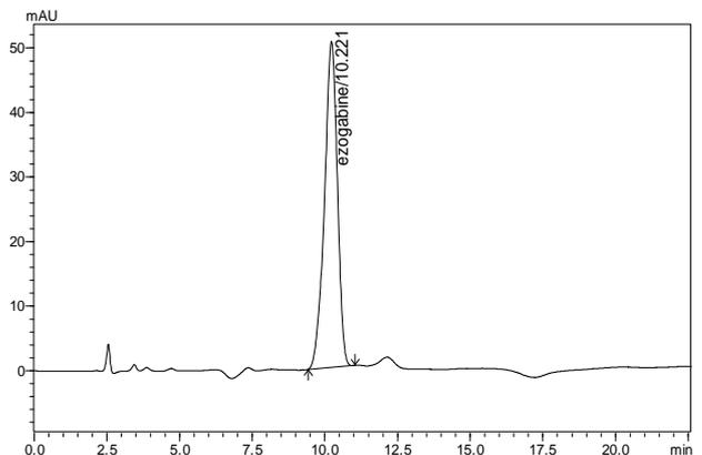
Figure 7: Thermal degradation chromatogram of Ezogabine
