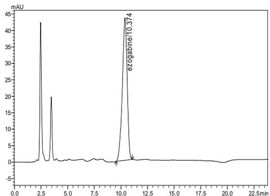
Figure 6: Peroxide (3% H<sub>2</sub>O<sub>2</sub>) degradation chromatogram of Ezogabine
