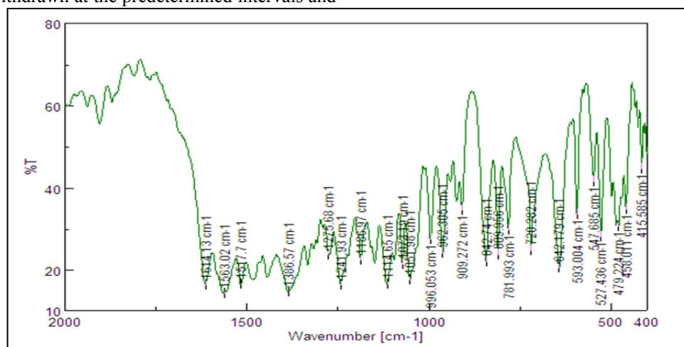
Figure 1: FT-IR spectra of Metoprolol Succinate (Obtained)
