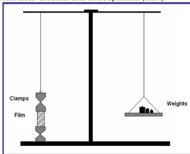
**Modified tensile strength tester.**
