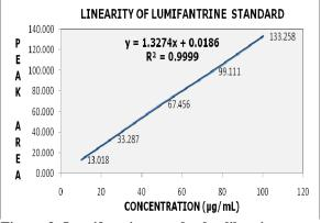
Figure-3: Lumifantrine standard calibration curve
