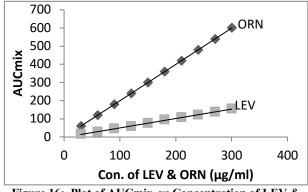
Figure 16: Plot of AUCmix vs Concentration of LEV & ORN with p-CA in dosage form
