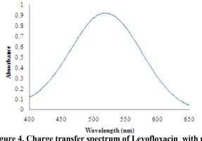
Figure 4. Charge transfer spectrum of Levofloxacin with p-CA
