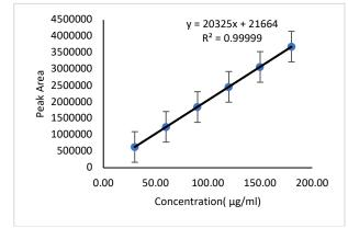
Figure 2:Calibration graph for Bedaquiline
