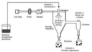
**Fig - 4: Microspheres by Spraying Drying Technique**
