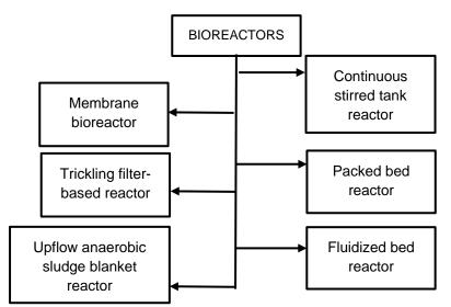
Fig 3. Various bioreactors used for biohythane production
