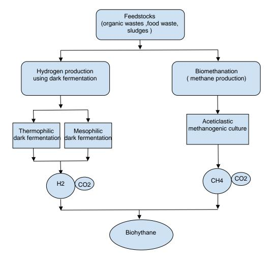
Fig 2. Outline of biohythane production procedure
