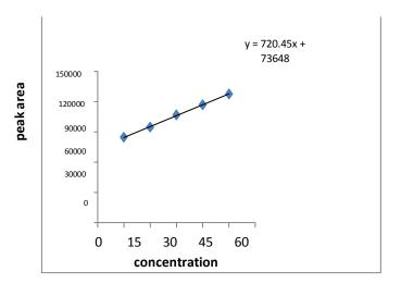
Figure X Calibration Curve of Tenofovir Disoproxil Fumarate(TDF)
