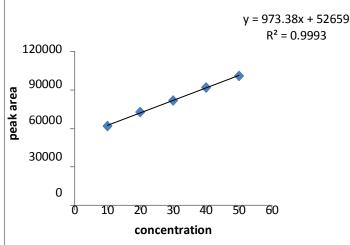
Figure IX Calibration Curve of Emtricitabine (EMT)
