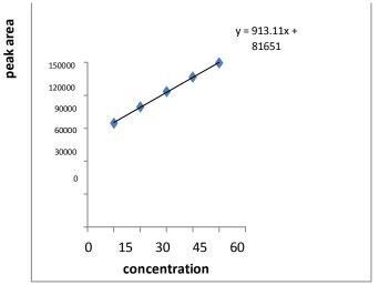
Figure XI Calibration Curve of Isoniazid (INH)
