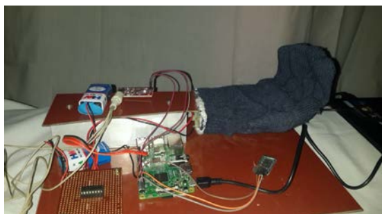
Figure 2: Grab Position of hand prototype in lateral view
