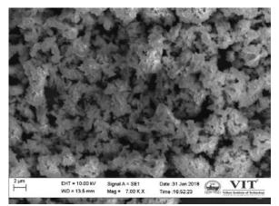
Fig 2.7. SEM image of silver-6-ABI surface complex
