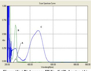
Figure (1) :( B) Arsenazo III Vs. distilled water. (A): Amoxicillin Vs. Distilled water. (C): Complex product Vs. Blank
