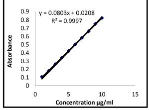
Figure (2): Calibration Curve for the determination of Amoxicillin.
