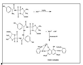
Scheme (3): The mechanism of oxidation of Amoxicillin
