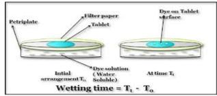
Fig 6: Wetting time of Mouth dissolving tablet. The time taken for appearance of dye colour on tablet is wetting time.
