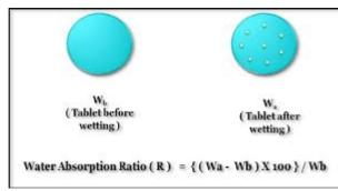
Fig 7: Calculation of water absorption ratio for MDTs. Difference between initial and final weights of tablet is noted Water absorption.
