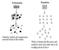
Fig. 3: Disintegration by Deformation and Repulsion
