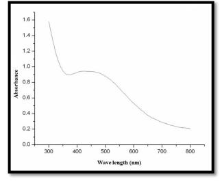
Figure (7):UV-Visible spectroscopy of silver nanoparticles produced by *F. graminurum*.
