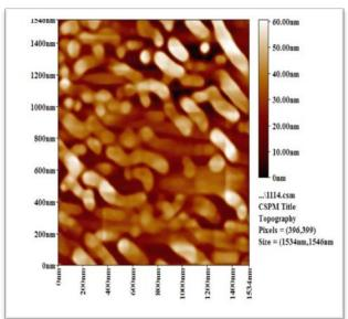
B Figure (3): AFM images of silver nanoparticles produced by *F. graminurum* (A) three dimensions 3D and (B) two dimensions 2D
