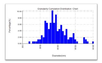
Figure(2):Granularity volume distribution chart of silver nanoparticles produced by *F. graminurum*
