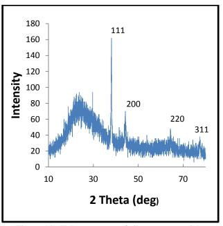
Figure (6): X-Ray pattern of silver nanoparticles produced by *F. graminurum*.
