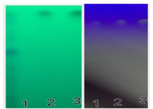
Fig.8: High-performance thin-layer chromatography plates for 1ethyl acetate fraction and 2-isolated3-standard quercetin detection under ultraviolet light (a) at 254 nm and (b)at 366 nm
