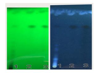
Fig.9: High-performance thin-layer chromatography plates for 1-nbutanol fraction and isolated3-standard apigenin, detection under ultraviolet light (a) at 254 nm and (b)at 366nm
