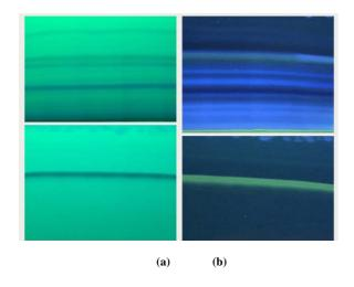
Fig. 6: Preparative thin-layer chromatography for standard quercetin (1) and ethyl acetate fraction (2) and on silica gel GF254, detection by ultraviolet light (a) at 254 nm and (b) at 366 nm
