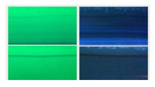
(a) (b) Fig. 7: Preparative thin-layer chromatography for standard apigenin(1) and n-butanol fraction (2) and on silica gel GF254, detection by ultraviolet light (a) at 254 nm and (b) at 366 nm
