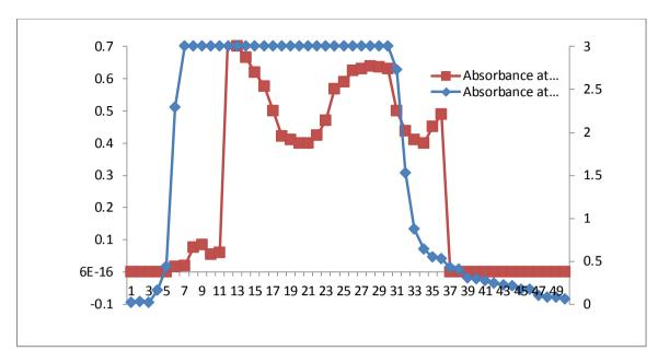
Figure 4 :Gel filtration chromatography (step 1) for purified biosurfactant from *Saccharomyces cerevisiae* by using Sepharose-6B column (1.5x80) cm. The column was calibrated with 0.1M PBS pH 7.2 ; flow rate 30 ml/hrs and 5 ml/fraction.
